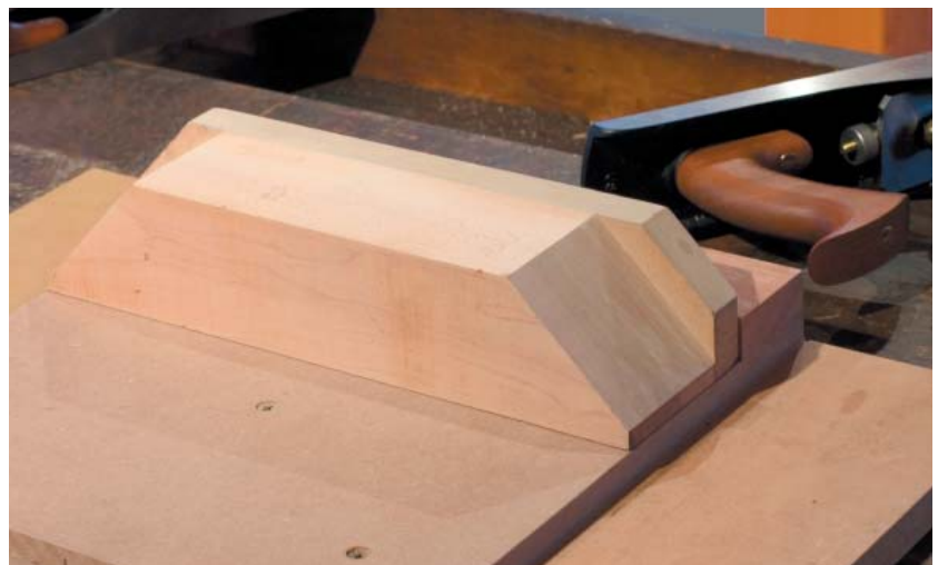
45° Miter 'Bird House' Fixture
